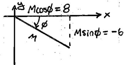
$$\therefore M = \sqrt{8^2 + 6^2} = 10, \quad \phi = \text{atan2}(-6/8) = -36.86^\circ$$
