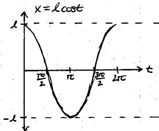
$$T = 2\pi \text{ seconds/cycle} \quad \dots \text{ period}$$
