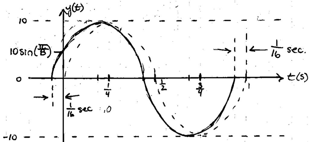
$$\theta = \omega t = \phi = \frac{\pi}{8} \Rightarrow t = \pi/8 / \omega = \pi/8 / 2\pi = \frac{1}{16} \text{ s}$$
