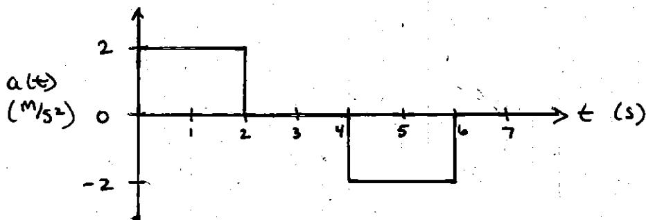
Knowing that the particle starts from rest and travels a total of 16 m, sketch graphs of the position  $x(t)$  and velocity  $v(t)$ .
