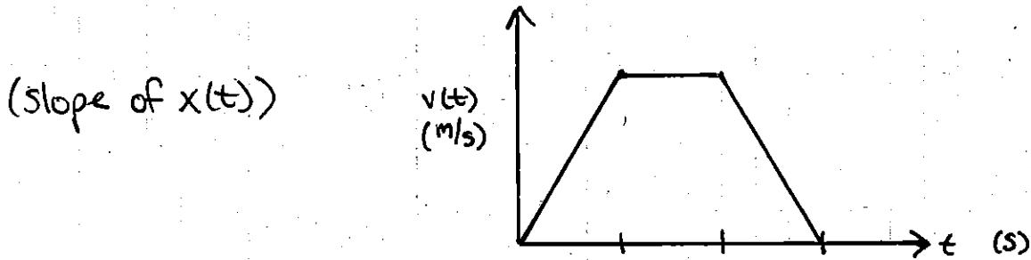
→ The acceleration  $a(t)$  is the instantaneous rate of change of the velocity:
