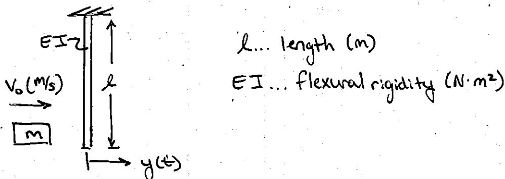
The resulting displacement of the cantilever is  $y(t)$ ,
