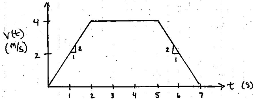
Now we can use graph of  $v(t)$  to construct  $x(t)$  knowing that the slope of  $x(t)$  is  $v(t)$ :  $\frac{dx}{dt} = v(t)$ .
