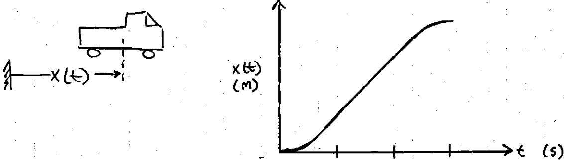
→ The velocity  $v(t)$  is the instantaneous rate of change of the position (ie, the derivatives):
