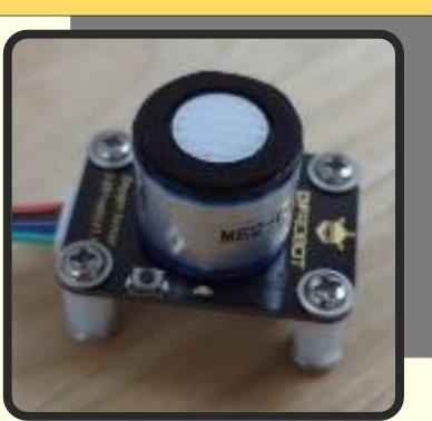
2.) Oxygen sensor detects a preset % O2 and shuts off the vacuum pump.
