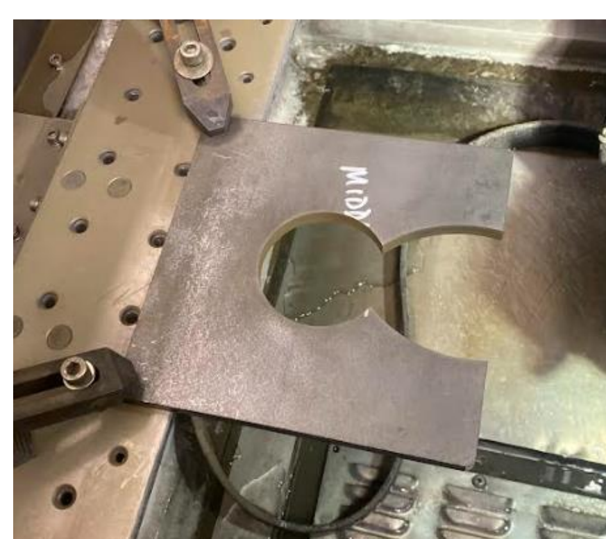
Machining of the (5) middle plates, each plate required two operations (Material Resources LLC)
