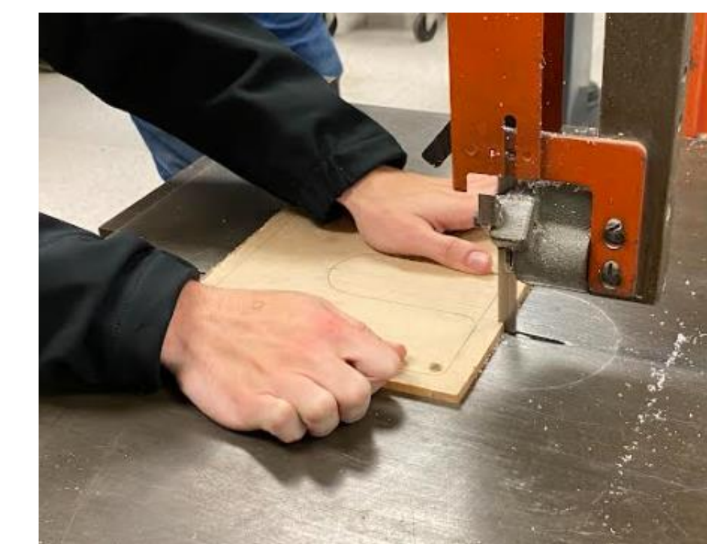
Cutting slot/ drilling holes in top plate (Wright State Lab)
