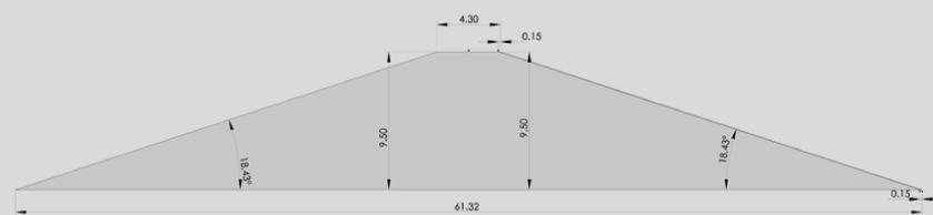
The dirt berm that makes up the walls of the reservoir requires a shallow 1:3 slope to ensure that it lasts a long time.
