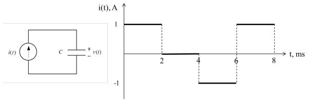
a) Knowing that  $i(t) = C \frac{dv(t)}{dt}$ , sketch the voltage across the capacitor v(t). Note that the time is measured in *ms* and the initial voltage is zero (i.e., v(0) = 0). (5 points)
