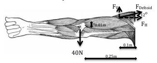
The horizontal  $F_H$  and vertical  $F_V$  components of the deltoid muscle force for the configuration shown above satisfy the following system of equations:
