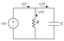
a) Given that  $i(t) = i_1(t) + i_2(t)$ , write i(t) in the form  $i(t) = M \sin(\pi t + \phi)$ (i.e., find M and  $\phi$ ). (10 points)
