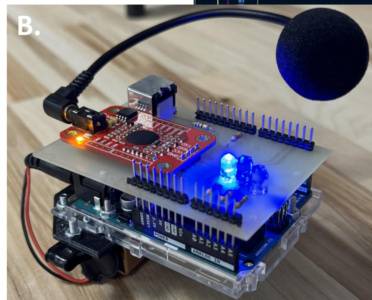
Figure 5B shows the completed stand-alone device when the PCB is plugged into the Arduino UNO with the microphone and powered via 9-volt battery.
