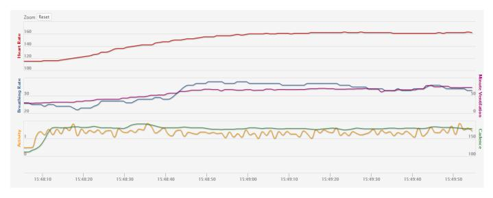
Figure 2. The Hexoskin data for a Run sequence showing the HR (top red), BR (blue middle), and A (yellow bottom) signals are labeled with the Y Axis on the left, and MV (purple middle), and C (green bottom) signals labeled with the Y Axis on the right. The X Axis represents time in the format hour : minute : second.
