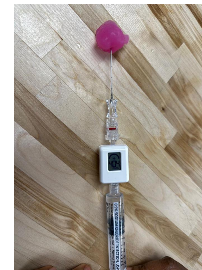
Image 4: Pressure Measurement During Injection into Silicone Tumor Phantom
