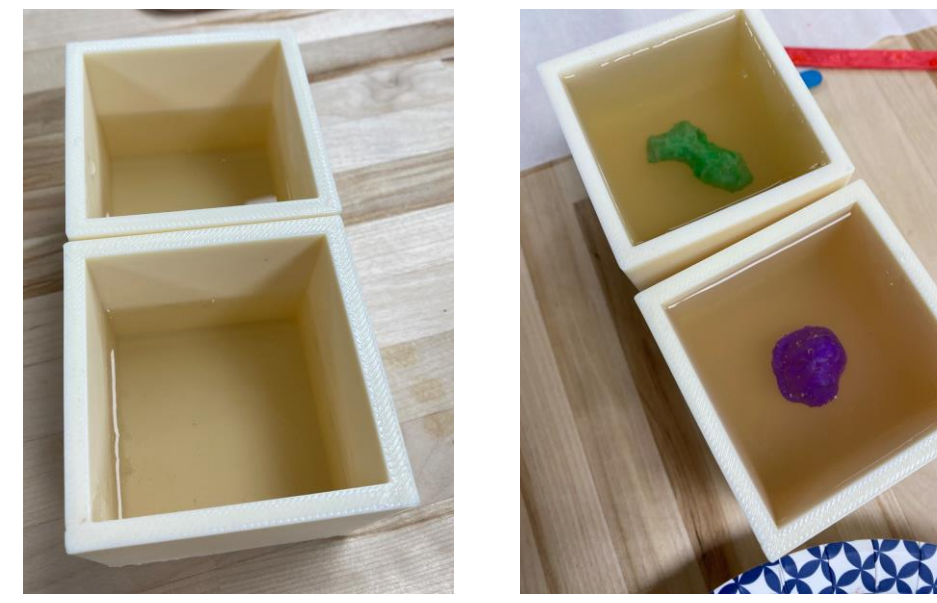
Image 1. Visual display for filling the box half-way with agar, allowing it to set, placing the permanent tumor model within the box on top of the agar, and filling the remaining space with agar to create one whole model.
